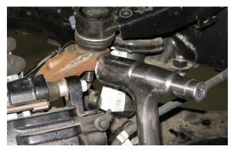
15. Break loose but do not completely remove the 27mm lower ball joint nut. Ensure there are few threads engaged to help unseat the ball joint. With a large hammer, strike the side of the spindle boss until the lower ball joint is dislodged.
