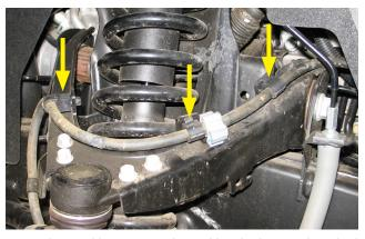
10. Remove the 15mm end link nuts to detach the end links from the sway bar and lower control arm. Use the hex stud on the ball joint to prevent the stud from turning while removing the nut.
