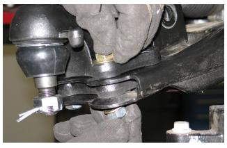
28. Mount the upper ball joint to the top housing hole on the spindle. Secure the ball joint with the mounting nut finger tight, but do not tighten.
