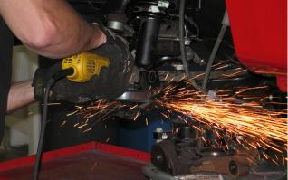
21. Use a grinder to smooth the cut surface. Wipe the area down with a cleaning solvent and spray paint the exposed metal.
