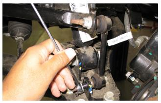
11. Break loose but do not completely remove the 21mm tie-rod ball joint nut. Ensure there are few threads engaged to help unseat the tie-rod ball joint.
