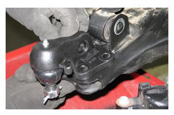
27. Fasten the lower ball joint assembly with four 7/16"-20 X 2.25" hex head bolts, four flat washers, and the four 7/16"-20 lock nuts supplied with the lower ball joint. Torque to 44 ft lbs.
