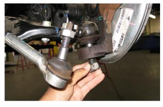
16. Remove upper and lower ball joint nuts to detach the spindle from the control arms.
