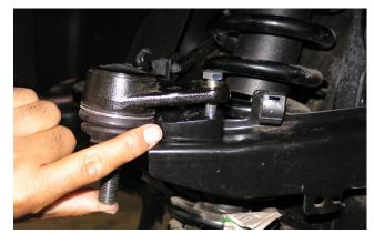
23. The bottom spacer is placed on the underside of the upper control arm.
